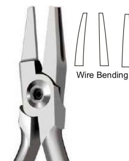
Aderer V-12-4912 12 cm/ 4¾" Three Jaw Plier, Aderer The precision aligned tips ensure for consistent bends. Gradually tapered for delicate bending. For wires up to 0.036" ( 0.91 mm )
