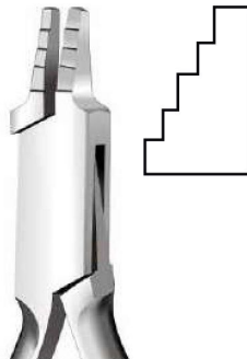
V-12-6612 Loop Closing Plier, Nance Style Box joint with 4 sectioned tip for forming various size loops in rectangular and round wires. For wires up to .028" ( 0.71 mm).
