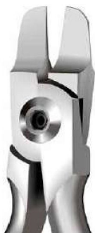
Tweed V-12-4611 T/C 11.5 cm/ 4½" Rectangular Arch Pliers, Tweed Style Forming plier for square or rectangular wires. The blades are designed to be parallel at .020" ( 0.51 mm ) opening. The working edges are carefully diamond-honed to prevent wire scoring.
