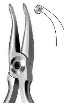
How V-12-5013 12.5 cm/ 4¾" Utility Plier , How Style With 1/8" ( 3.2 mm ) gripping pads, which are serrated to hold wire securely. Beaks are completely lip safe.
